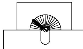
The locking lever should be in the OPEN position at this time. The boltwork is not blocked as long as the locking lever is in the OPEN position and the vault may be locked and unlocked by its normal locking means as necessary.
